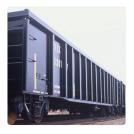
**Gondolas**: Open-top cars used for scrap metal, gravel, or coils.
