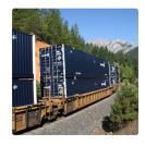
Well Cars: Designed to carry intermodal containers. The lower center of gravity helps with speed and safety.
