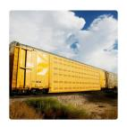
Autoracks: Also called a multilevel carrier, this railcar is an enclosed or partially enclosed railcar used to move new automobiles, SUVs, trucks, and vans from manufacturing plants to distribution centers. They're designed to protect vehicles from weather, theft, and damage in transit.
