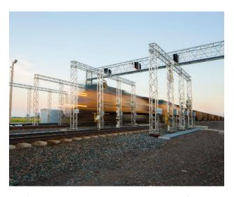
Machine visioning can take 1,000 images per rail car at speeds up to 70 mph, identifying defects early for maintenance.
