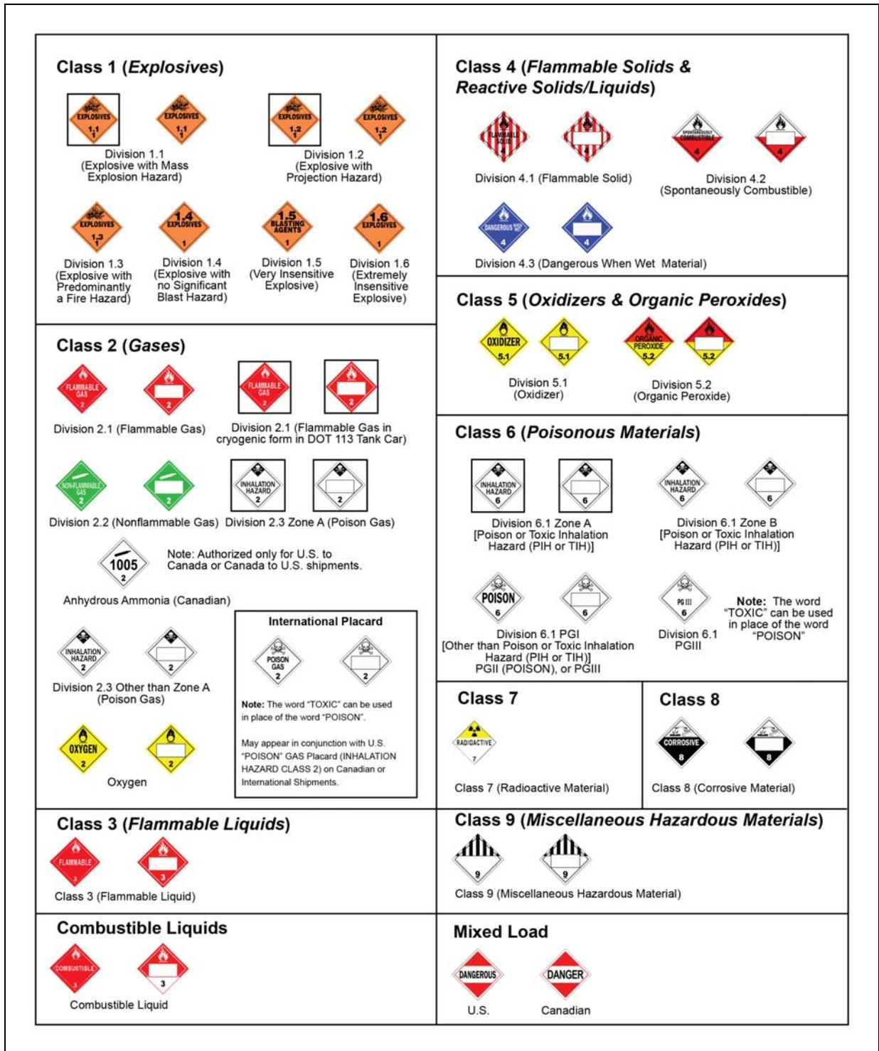
**Figure 4. Placards for Hazardous Materials by Hazard Class**
